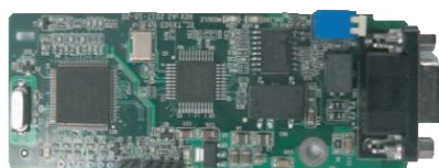
PROFIBUS-DP communication card EC-TX503
