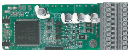
24V incremental PG card EC-PG505-24
