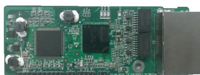
PROFINET communication card EC-TX509
